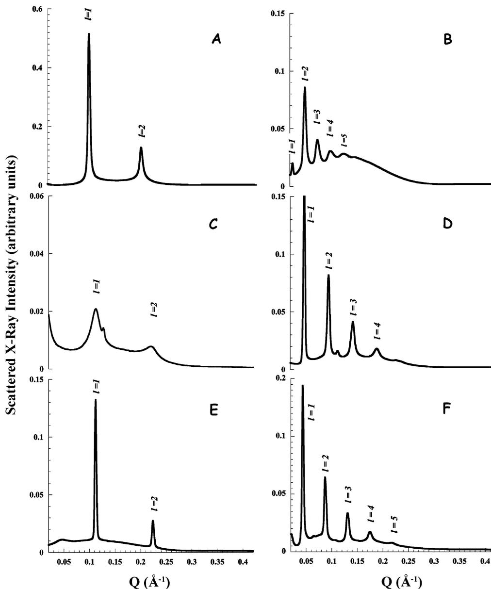
**Figure 2.** Synchrotron small-angle X-ray scattering profiles collected for (A) 30 wt % DMPC dispersion in water and for quaternary mixture employing (B) 10 mol % PEG5000–DMPC conjugate, (C) 10 mol % F38 polymer, (D) 10 mol % F88 polymer, (E) 10 mol % F68 polymer, and (F) 10 mol % F98 polymer. All measurements were made at 37 °C.
