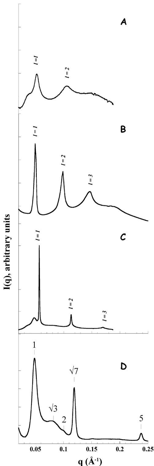
**Figure 4.** Synchrotron small-angle X-ray scattering profiles collected for quaternary mixture prepared with increasing concentration of PEO–PPO–PEO triblock copolymers: (A) 4 mol % F98; (B) 8 mol % F98; (C) 12 mol % F98; (D) 20 mol % F98. All measurements were made at 37 °C.
