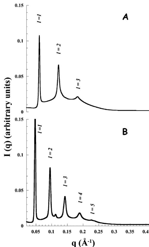
**Figure 3.** Synchrotron small-angle X-ray scattering profiles collected for quaternary mixture prepared with PEO–PPO–PEO triblock copolymers (A) 10 mol % P85 and (B) 10 mol % F88. All measurements were made at  $37 \text{ }^\circ\text{C}$ .
