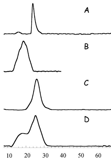
**Figure 5.** Calorimetric scanning curves: (A) DMPC dispersion in water; (B) 10 mol % PEG5000-grafted lipid-based complex fluid composition; (C) 10 mol % F68 Pluronic-based complex fluid composition; (D) 10 mol % F98 Pluronic-based complex fluid composition. Heating rate was 5 °C/min.
