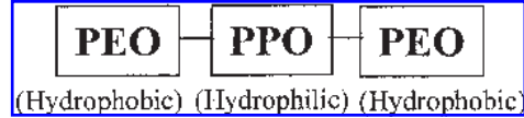
FIG. 3. The molecular structure of Poloxamer 188 (P188). It has an amphiphilic, tri-block copolymer structure. This water-soluble surfactant contains a central hydrophobic block of polypropylene oxide (29 PPO) moieties and two peripheral hydrophilic blocks of polyethylene oxide (38 PEO) moieties.
